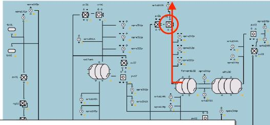
• "Diagnosis can decide whether the venting valve VR01 is closed or stuck open (assuming no other failures)"
