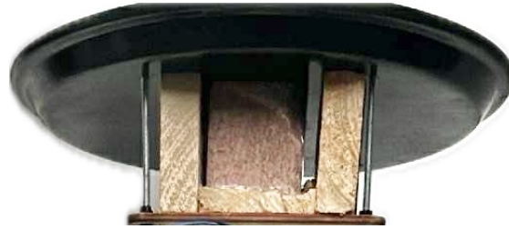
Figure 5.13: Side view of the top part of the robot. It is composed of a rounded plate and a counterweight.
