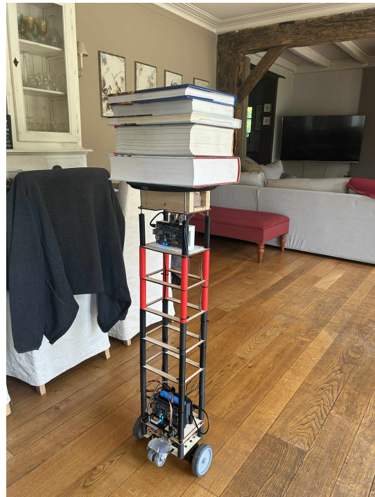
(b) Picture of the robot during the test with 14 kg of payload.
