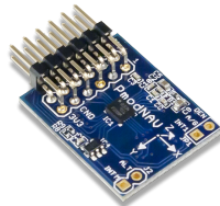
Figure 2.2: Top view of the Pmod NAV sensor [13].
