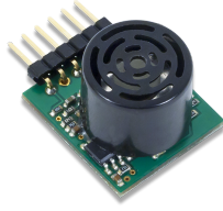
Figure 2.3: Top view of the Pmod MAXSONAR module used for ultrasonic distance measurement [14].
