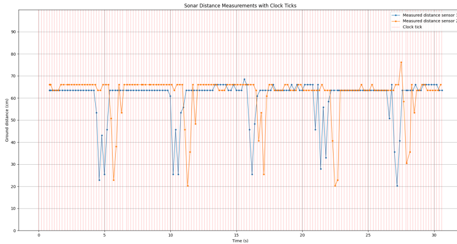
Figure 5.1: Sonar Measure Without Acoustic Foam
