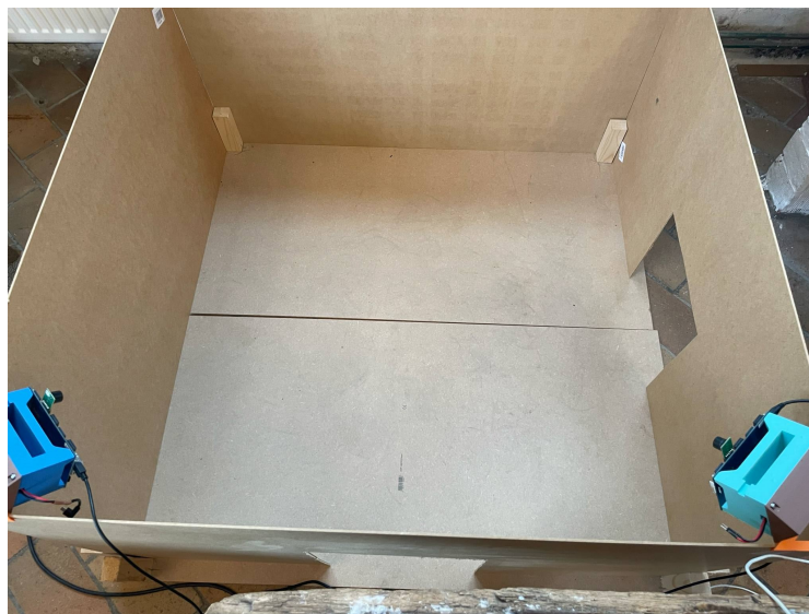
Figure A.3: Room setup with no absorption
