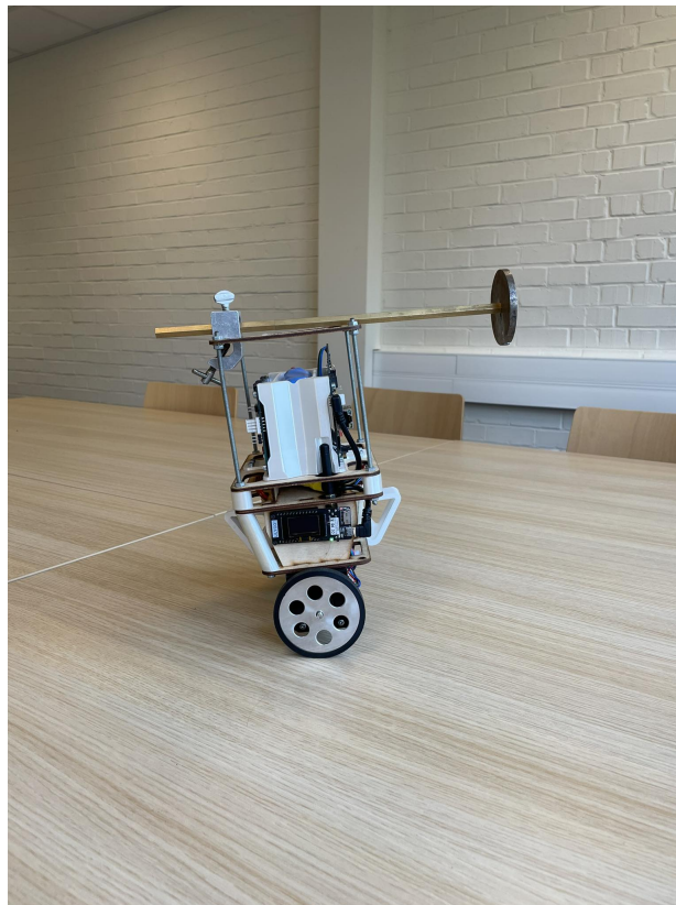
Figure H.1: Picture of the robot during the offset mass test.
