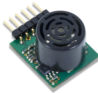
Figure 4.: Pmod MAXSONAR: Maxbotix Ultrasonic Range Finder.
